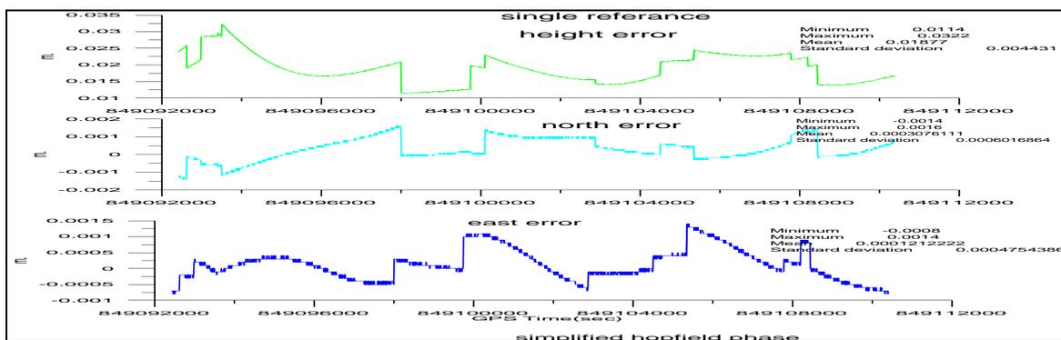
Figure (2): The differences between the default code- phase solution and the code-phase solution by replacing the troposphere model to *Simplified Hopfield* at Mecca network
